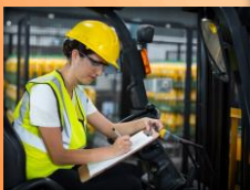
Inspect the lift prior to elevating employee
