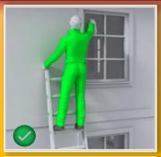
Correct – user maintaining three points of contact (means of securing omitted for clarity)
