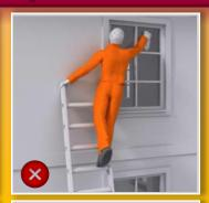
Incorrect – overreaching and not maintaining three points of contact
