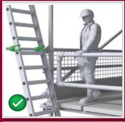
Correct – access ladders should be tied and extend at least 1 m above the landing point to provide a secure handhold
