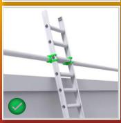
Correct – ladder tied at top stiles (correct for working on, but not for gaining access to a working platform/roof etc)
