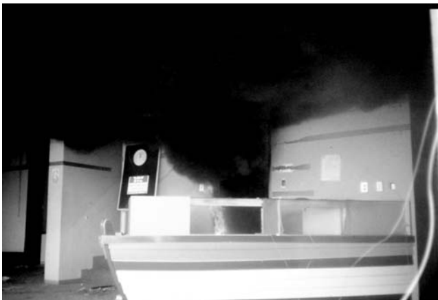
Figure 9.1 Outflow of smoke through the upper part of an opening in a compartment fire.
