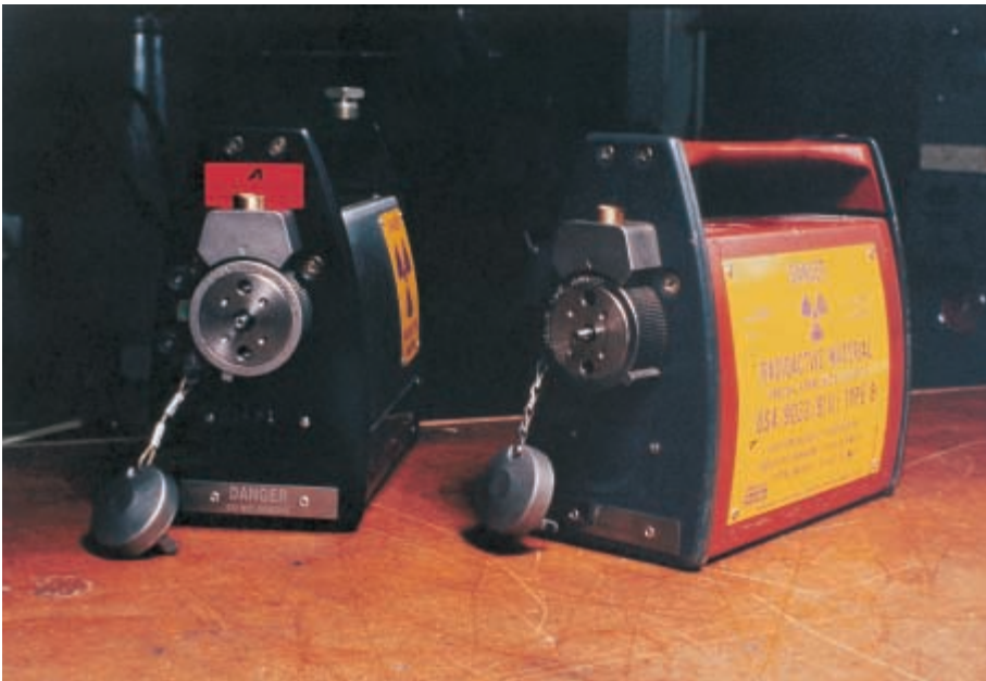
FIG. 2. Class P portable exposure device.
