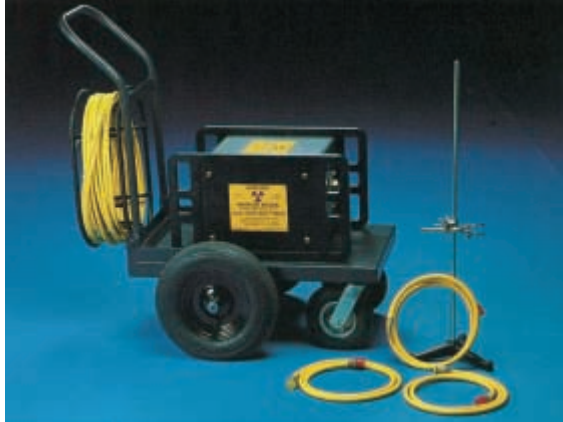
FIG. 3. Class M mobile exposure device.
