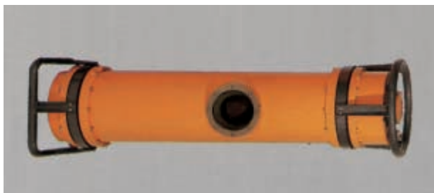
FIG. 8. Direct radiating portable X ray tube assembly.
