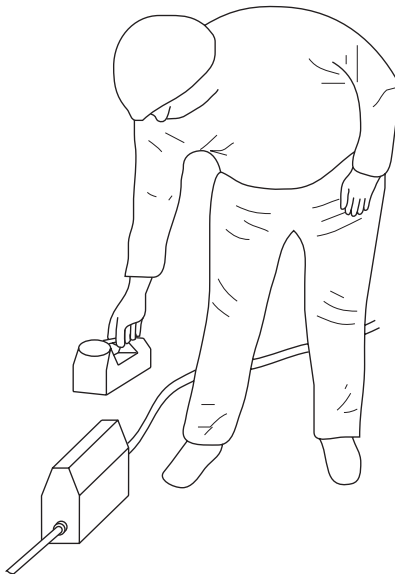
FIG. 15. Use of instrument to survey an exposure device.
