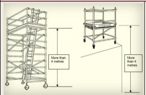
Persons using the mobile scaffold must be trained in the safe erection use and dismantling of the scaffold.
