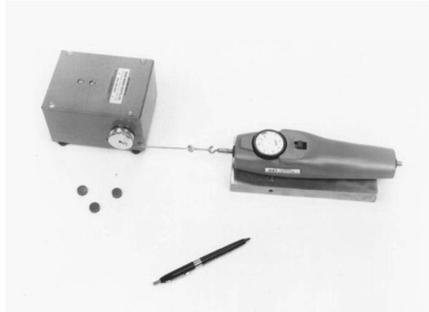
FIGURE 12.9 Horizontal pull slipmeter (HPS). (From Chang, W.R. et al., Ergonomics , 44, 1233–1261, 2001.)
