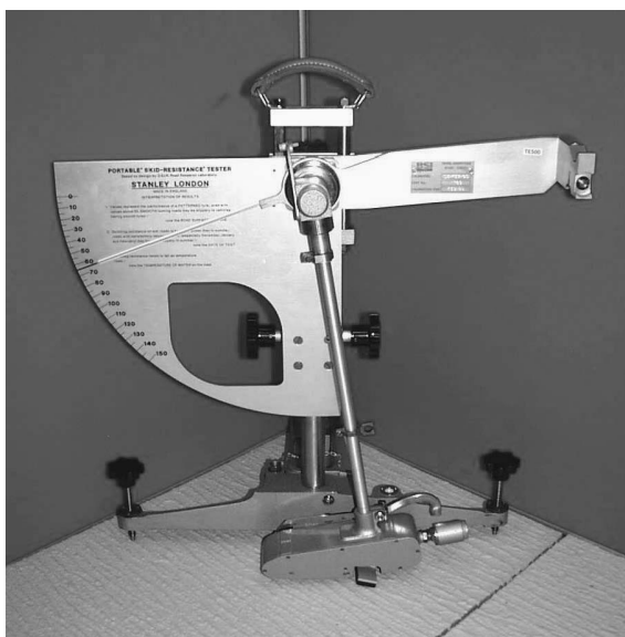
FIGURE 12.17 British portable skid tester (BPST). (From Chang, W.R. et al., Ergonomics , 44, 1233–1261, 2001.)
