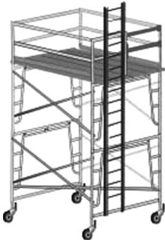
FIGURE 31.8 Manually propelled mobile scaffold. (Source: Occupational Safety & Health Administration, Washington, DC.)
