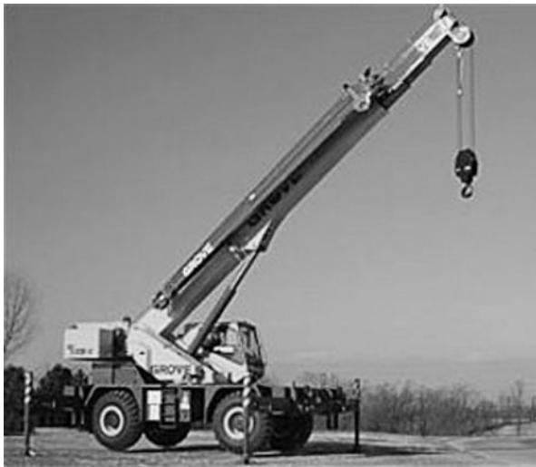
FIGURE 23.17 Rough-terrain, wheel-mounted crane, telescoping boom. (Source: GROVE, Manitowoc Cranes, Manitowoc, WI)
