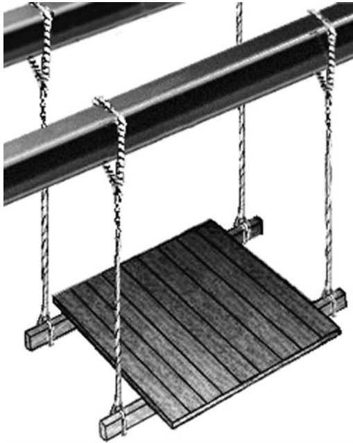
FIGURE 31.3 Interior-hung scaffold. (Source: Occupational Safety & Health Administration, Washington, DC.)
