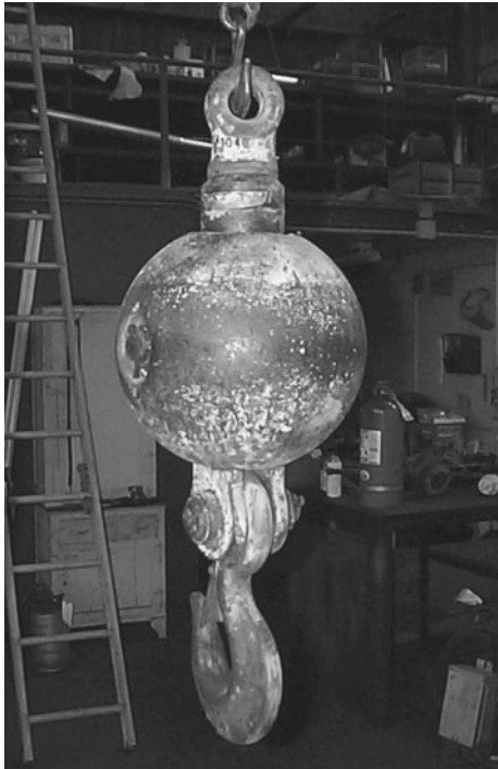
FIGURE 16.17 Typical swivel and headache ball, attached to hook. (Source: Gunnebo Johnson Corp., Tulsa, OK.)
