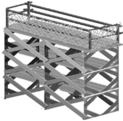
FIGURE 31.5 Bricklayer’s square scaffold. (Source: Occupational Safety & Health Administration, Washington, DC.)
